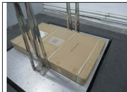
Block 12 Face 3 (Pick-Up) Test Set up
