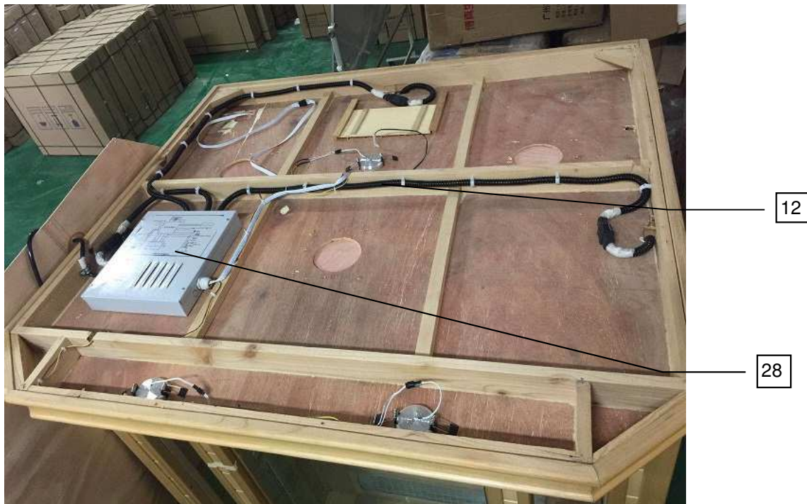
Photo 10 - Top View (Note: All wire to heaters are enclosed by metal conduit. A wooden cover enclosed all parts on the ceiling, which is fixed by screws)
