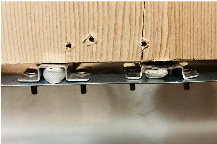
Photo 18 - Heater (Note: the thermostat & thermal link are fixed by Metal sheet & sleeving)
