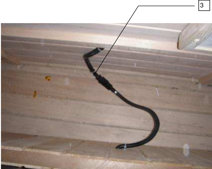
Photo 16 - Cord and Connection under seat, which cannot be contact without aid of tool
