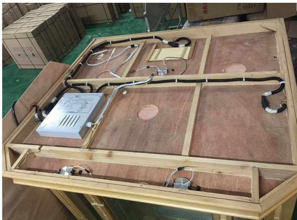
Photo 10 - Top View (Note:All wire to heaters are enclosed by metal conduit. A wooden cover enclosed all parts on the ceiling, which is fixed by screws)
